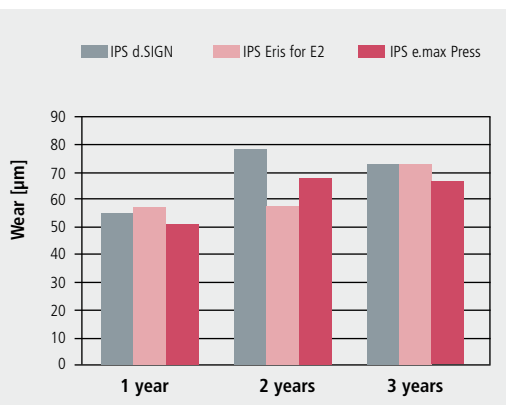
Fig. 29: Antagonist abrasion in relation to the wear period
